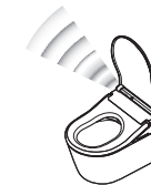
Body sensor A (Detects changes in heat)
